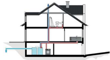
Installation utan tank i mark
